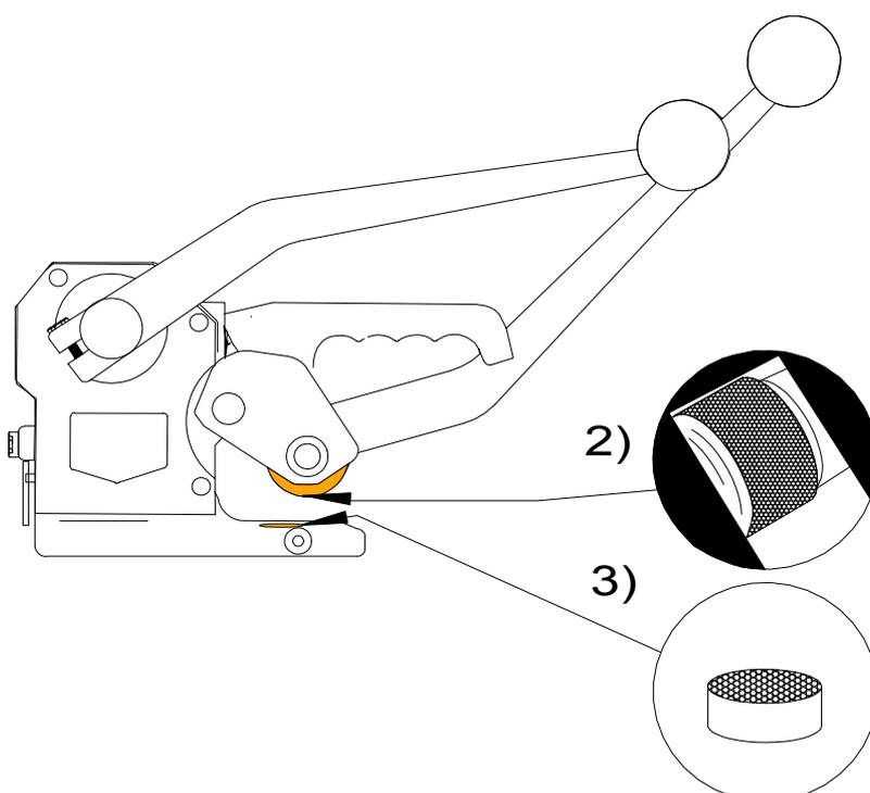
**E** Clean any swarf and dirt off the tensioning wheel (2), either by compressed air or with a small wire brush. Clean the pressure button at the same time.
