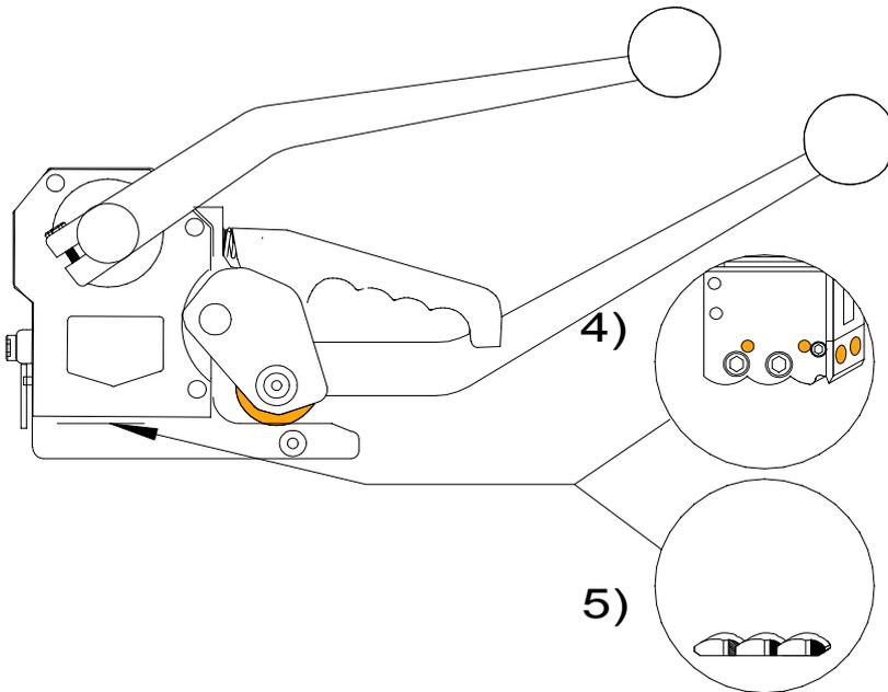
**E** Clean any swarf and dirt off the upper (4) and the lower punch (5), either by compressed air or with a small wire brush.
