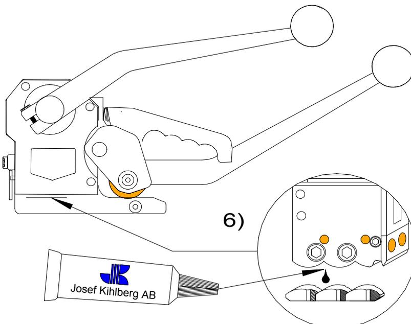
**E** Apply a little shearing oil (Nr 189323) to the surfaces of the punches (6) and then operate the strapper a few times without any strapping.
